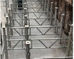
Alulight Props are lightweight aluminium props that come in a variety of sizes to enable many different propping heights up to and above 12 metres. This means ease of handling and speedy erection of support falsework.
