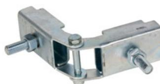
A small and simple device to fasten Steel Mesh Barriers together. The Steel Mesh Barrier Hinge will also allow easy access. Corners can be created at any angle between 76° and 284° when attached to the end of the barriers, but can also provide angled corners at any position along the barrier.
