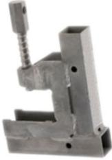
A small stable clamp attachment for steel. It can be mounted on the flanges of large steel beams, plate girders, or directly to flat plates like road plates. Grips to steel between 10mm and 50mm thick. It can be used vertically or horizontally.
