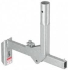
Used to provide a post attachment at an adjustable offset, up to max. 350mm from a vertical surface. Used in beam webs, on walls, façades, shaft sides, or slab edges etc. The bolt is pre-fitted to the base material and the keyhole used to initially secure the attachment until the fastener is tightened.
