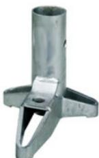
Used for horizontal surface applications, most commonly at the slab edge. The three points of support allow accurate installation on an uneven surface and ensure that the anchor load is correctly controlled. The Multi Foot can be through fitted using a variety of anchors appropriate to the base material.
