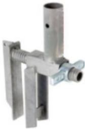
An attachment that clamps to narrow members from 0-150mm thick like steel sheets. This clamp also has reversible jaws. The heavy-duty coarse thread is quick to set, and tightened using a hammer. It is also robust to withstand site treatment. Can be mounted both vertically and horizontally.
