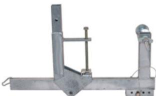
An adjustable Eaves Attachment for roof edge protection. The bolt accommodates large variations in the width of the support and the adjustable post holder allows flexibility in positioning.
