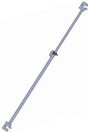
Adjustable braces for internal use in support structures, connecting to the horizontal Cuplok members. The overall length of the brace is set before installation by positioning the locating pin on the clamp in the appropriate hole and tightening the nut. Braces are available in two sizes which cover the various grid dimensions. See table below.
