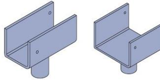
Designed to hold aluminium, steel or traditional timber beams. Forkheads are used in conjunction with the Universal Jack to give height adjustment. Nail holes are provided to allow timber beams to be fixed in place.
