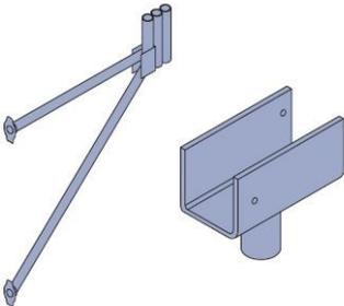
This bracket is designed for supporting cantilever edge slabs and incorporates 3 Jack locations at centres of 1.2, 1.25 and 1.3m. All jack locations can be utilised for traditional primary timbers.
