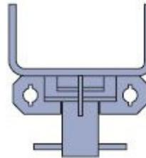
Forkheads for supporting slabs with slopes in one or two directions. Secondary sloping is achieved by rotating the small handles on the socket at the bottom of the forkhead. Incorporates a facility for jack bracing.
