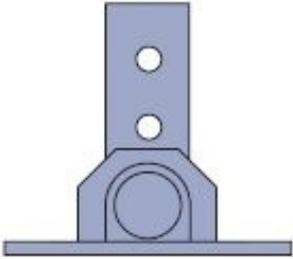
To support standards on sloping ground to a maximum of 45° from the horizontal. It should always be secured to a sound timber sole plate.
