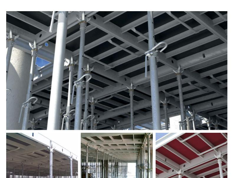
Airodek is a high-efficiency, low-weight slab falsework system, ideal for slabs up to 700mm thick. Designed for rapid assembly, one operative can set up as much as 40m2 per hour, dramatically cutting down on both time and labor costs.
