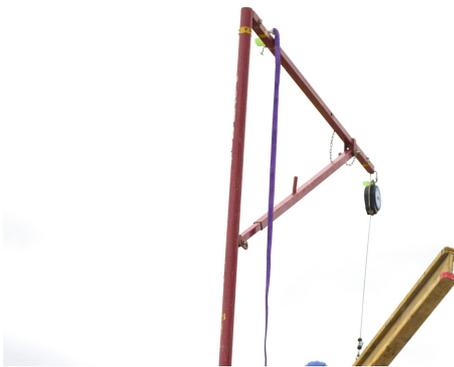
Designed for columns spaced up to 8.5m, allows the worker to safely cover a surface up to 125m<sup>2</sup> and a radius of 6.5m.
