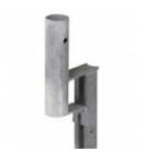
Used to support systems on stairs, permitting access to both the top surface and the soffit. Two spurs/studs are pushed into the concrete during installation stabilising the single point fixing. The Safety Post is positioned 90mm off the edge of the stairs, creating space for finishes and nosings.
