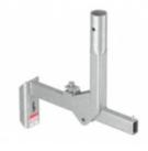
Used to provide a post attachment at an adjustable offset, up to max. 350mm from a vertical surface. Used in beam webs, on walls, façades, shaft sides, or slab edges etc. The bolt is pre-fitted to the base material and the keyhole used to initially secure the attachment until the fastener is tightened.
