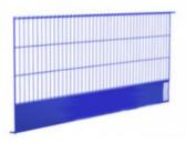
Lightweight, versatile barrier that provides hard-mesh coverage with impact-absorbing capacity. Each weld can withstand a force of 500kg. Designed with closed return for greater debris containment, and with reinforced edges to prevent site damage. Guardrails, toeboard and debris mesh in one product.
