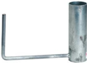
Accessory to the Multi Clamp to hold the clamp in place on the angled soffit of the stairs. The tube is fitted to the clamp's lower leg, and the hook engages on the step riser. This restrains the clamp assembly.
