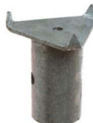
The Soffit Grip is placed on top of the upper post and firmly secured with a clip. When compressing the post against the soffit, the spikes apply a firm grip preventing the system from sliding in case of accident or severe weather conditions.
