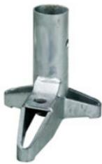
Used for horizontal surface applications, most commonly at the slab edge. The three points of support allow accurate installation on an uneven surface and ensure that the anchor load is correctly controlled. The Multi Foot can be fitted using a variety of anchors appropriate to the base material.
