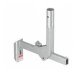
Used to provide a post attachment at an adjustable offset, up to max. 350mm from a vertical surface. Used in beam webs, on walls, façades, shaft sides, or slab edges etc. The bolt is pre-fitted to the base material and the keyhole used to initially secure the attachment until the fastener is tightened.
