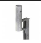
Used to support systems on stairs, permitting access to both the top surface and the soffit. Two spurs/studs are pushed into the concrete during installation stabilising the single point fixing. The Safety Post is positioned 90mm off the edge of the stairs, creating space for finishes and nosings.
