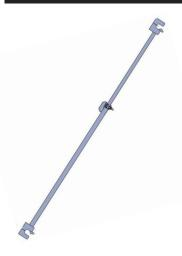
Adjustable braces for internal use in support structures, connecting to the horizontal Cuplok members. The overall length of the brace is set before installation by positioning the locating pin on the clamp in the appropriate hole and tightening the nut. Braces are available in two sizes which cover the various grid dimensions. See table below.
