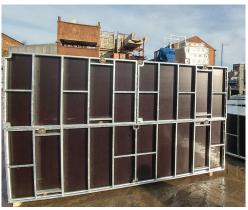
Easiform Frami Formwork is a man handleable formwork system that is perfect for foundations, bases and walls. The system has a robust galvanized frame and a safe working load of 50kN/M<sup>2</sup>.
