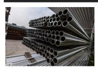
This tube has an outside diameter of 48.3mm, a wall thickness of 4mm, weighs approx. 4.37kg/m (1.36Kg/foot), is finished hot dip galvanised and is supplied fully certified to BS EN 39
