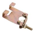
The Ladder clamp Double sided (Square edge) are supplied BS1139 and suitable for a wide range of Steel Scaffold Ladder types due to the double sided nature of the fitting.
