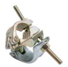
Supplied to EN74-1, Class B Specification, our Prop Bracing Double Coupler is used to fix Scaffold tube to Adjustable props as a means of bracing at 90Degrees.
