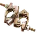
Scaffold Swivels are used on scaffold structures to join Scaffold Tubes at any angle, through 360. Most commonly when bracing is required throughout the scaffold structure. Pressed steel construction with a zinc plated exterior for long life.
