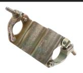
Supplied to BS1139, Scaffold Roofing Couplers are used to secure CI Sheets (sometimes referred to as Wrigley tin/corrugated sheets) to scaffold tube when construction a temporary or semi permanent roof structure with Scaffolding Tube and Scaffold Couplers.
