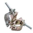
Supplied to EN74-1, Class B Specification, Prop Swivel Scaffold Fittings are used to fix Scaffold Tube to Adjustable Props as a means of bracing the Adjustable props with Scaffold tube at varying angles, through 360 degrees.
