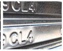
S235JRH graded steel produced in accordance to EN 10210-1 standards
